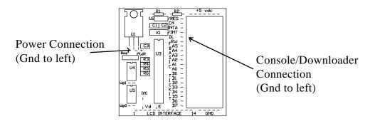
The above diagram shows the locations of components and pins for the TICkit. One important point to notice, is that the data group of outputs is numbered in the opposite order from the address group pins. This is simply a placement issue, but there is a possibility of confusion when wiring components to the TICkit.
