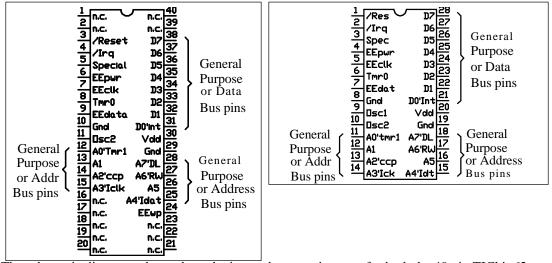
The schematic diagrams above show the internal connections are for both the 40 pin TICkit 62 module (on the left) and the TICkit 62 interpreter IC (on the right). The interpreter IC is available in both a 28 pin PDIP and 28 pin SOIC package.
