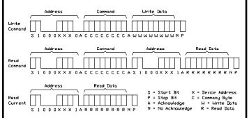
This command protocol is accomplished in FBASIC with the i2c\_write and i2c\_read functions. Both functions require a word parameter where the high byte is the address and the low byte is the command. The i2c\_read function returns the byte sent from the Xtender. The i2c\_write function sends the second parameter to the Xtender.
