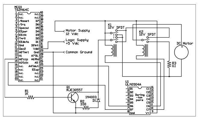
The following program illustrates these types of controls. The program sets up the PWM, turns the motor on at half speed and rotates it forward for 1 second, removes power and brakes the motor for 3 seconds, reverses direction and powers the motor at 1/4 speed for 2 seconds, removes power and lets the motor coast for 6 seconds, then repeats the
