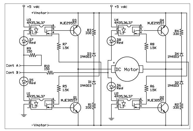
The solid state equivalent of the relay and PWM transistor is called an 'H' bridge. A schematic for a working H-bridge is shown above. The resistor values were selected for a 12 volt motor @ 2 amp max. If contA and contB are at the same logic level, the motor is not being driven. If contA is low and contB is high, the motor spins forward. If contA is high and contB is low, the motor spins in reverse.
